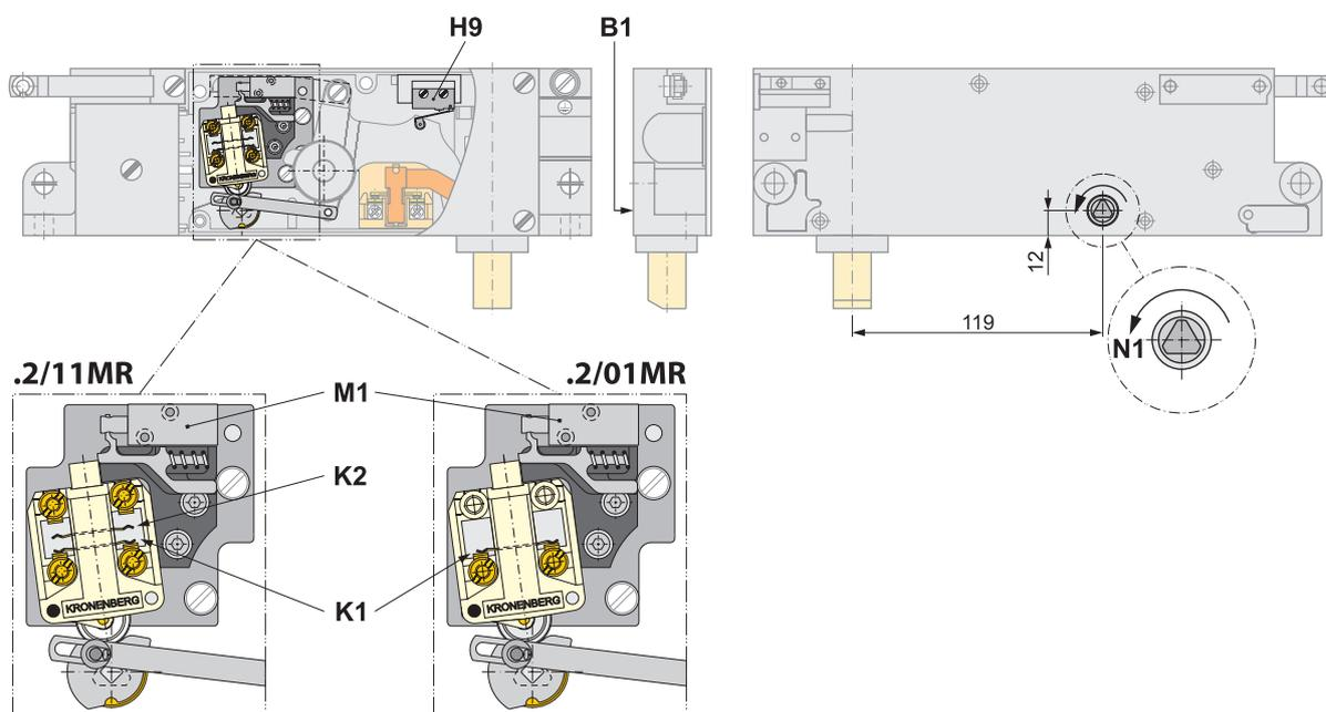
K1 Zwangsöffner / *positively driven normally closed contact*
